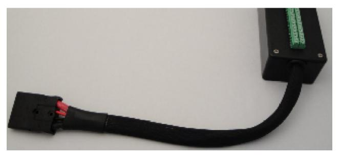
**FIGURE 16.10.2.** Dynapulse 24-Input Temperature Monitoring Block showing connection for Dynapulse™.
