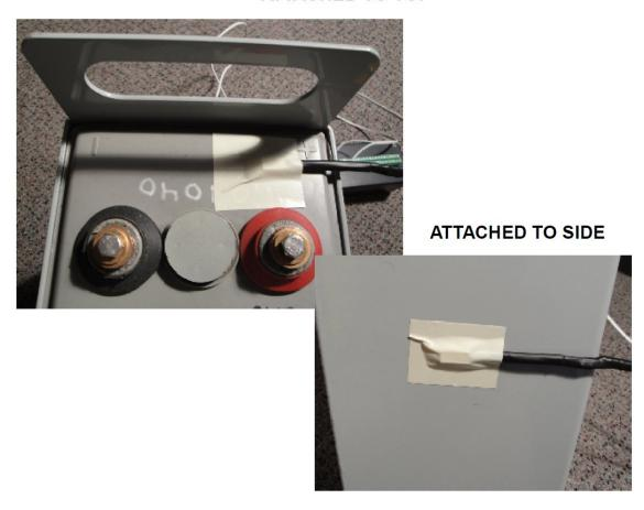
**FIGURE 16.10.7.** Temperature switches showing connections to TOP and SIDE. Up to 24 locations may be used.
