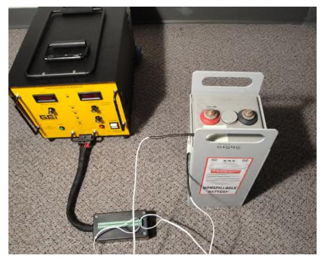
**FIGURE 16.10.6.** Temperature switches connected to battery in two locations.
